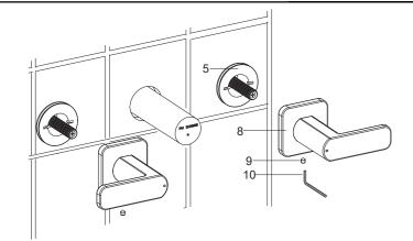
Place the handle kits(8) onto the escutcheon bases(5) with the valves closed.
