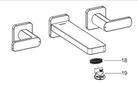
Ensure that all coupling nuts are tight. Ensure that the handles are in the off position. Turn on the main water supply and drain, and check for leaks. Repair as needed.
